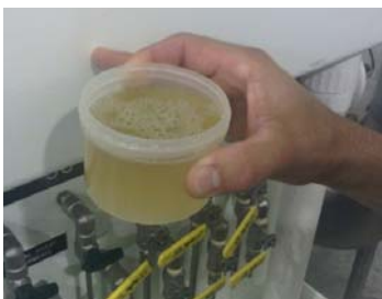
Figure 3 Highly Colored Feedwater of the Pompano Beach Plant
